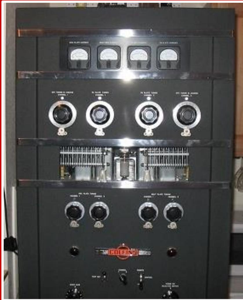
“This 250 watt commercial AM transmitter was a brother of the famous 30K-1 amateur AM transmitter. This rig features beautiful audio, the option of using audio clipping, and dual 75THs modulating a 4-125 driven by an 807. The 30K-5 is a two channel transmitter.”
