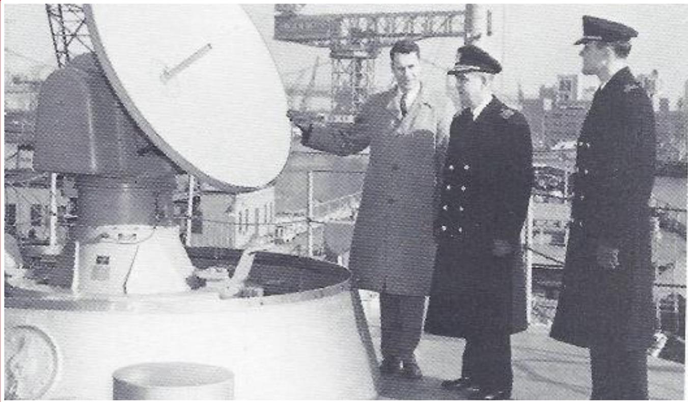
“The ship’s navigator can find his position just as if he had an assistant watching the sun through an ordinary sextant. No cloudy weather gets in the way of the radio sextant, nor can an enemy jam the radio impulses (as is possible with other radio aids to navigation, such as Loran.”
