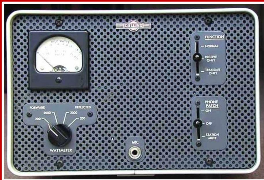
STATION CONSOLE – directional coupler, wattmeter, speaker, phone patch, interconnections.
