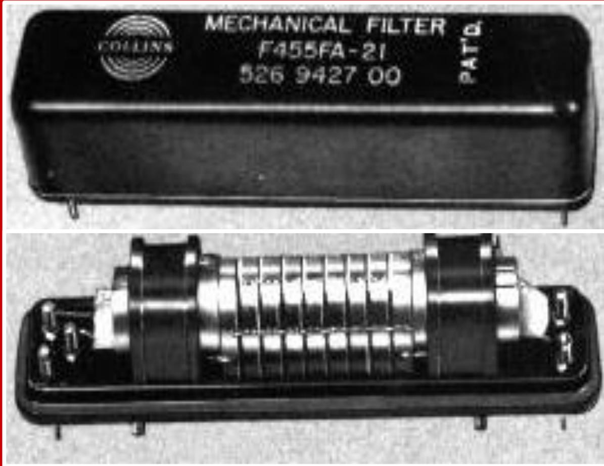
“The filter is a mechanically resonant device which receives electrical energy, converts it into mechanical vibration, filters out unwanted frequencies, then converts the mechanical vibration back into electrical energy at the output.
