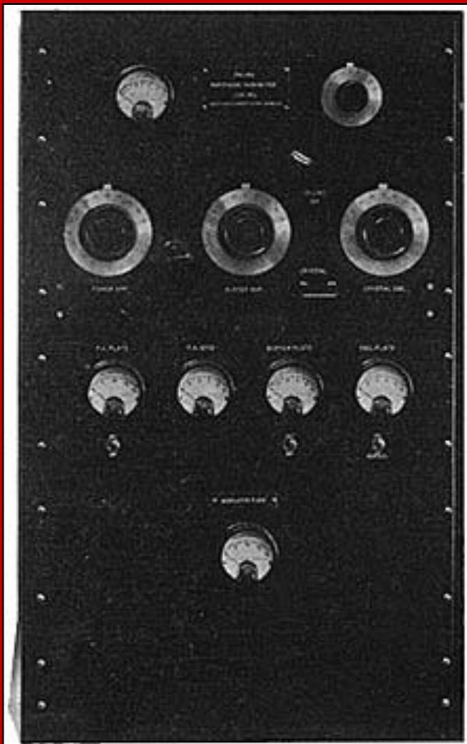
The 40A/B was Collins' first desktop phone transmitter. Based on the 30W, it added a 9C amplifier-modulator and antenna tuner unit. Plug-in coils for 160, 80, 40, and 20 meters were available
